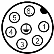
X 2: Connector S1/S2 (Rotary potentiometer for actual value feedback)
